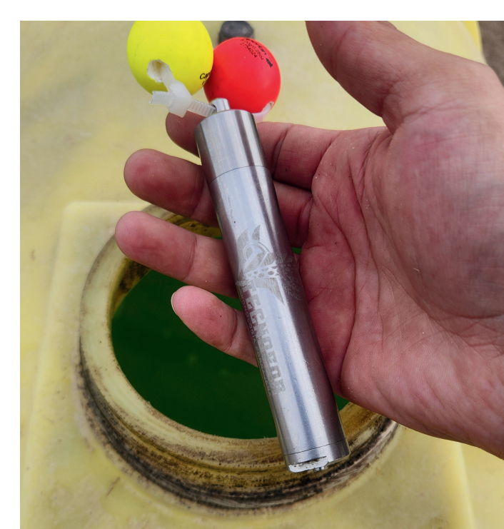
Figure 2. Data loggers, programmed to record temperature every 5 minutes, were placed in the inoculant tank.
